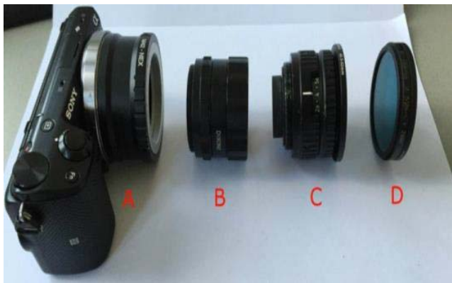
Figure-2. Camera system for the Setup-II. (A) converter ring, (B) extension ring, (C) lens (D) filters and UV imaging Setup-II
