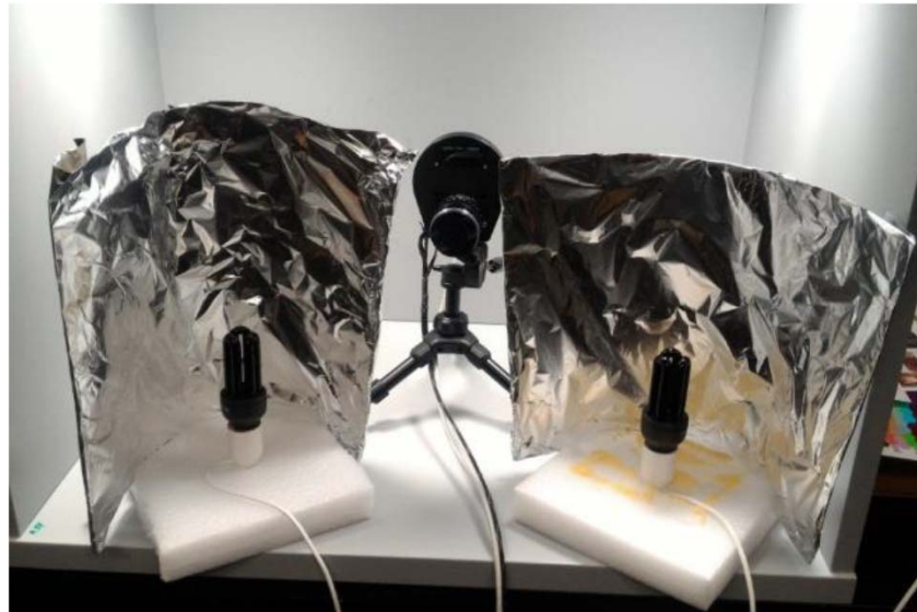
Figure-1. Setup-I utilizing PIXELTEQ's SpectroCam Multispectral Camera
