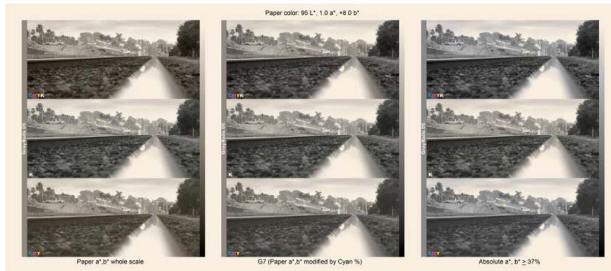
Three different Gray Balance formulae on yellow-biased paper.
