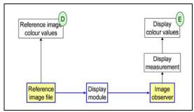
Methods for assessing colour accuracy and other image attributes for an end-to-end test (A compared to C), for an image capture module test (A compared to B) and for the display module test (D compared to E) are described.
