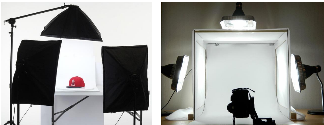
Figure 1. Example of diffuse lighting setups using commercial softbox lighting (left), or a homemade lightbox with diffuse walls (right).
