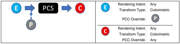
In this scenario a profile conforming to this ICS is used as a source profile with a colorimetric PCS connected to an arbitrary profile that is set up to use a colorimetric PCS. The transform type for profile E is "colorimetric" indicating that the transform from an AToBxTag from profile E is used to transform device values to a colorimetric PCS.
