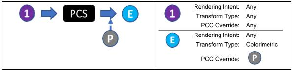
In this scenario an arbitrary profile is connected to a profile conforming to this ICS used as a destination profile.
