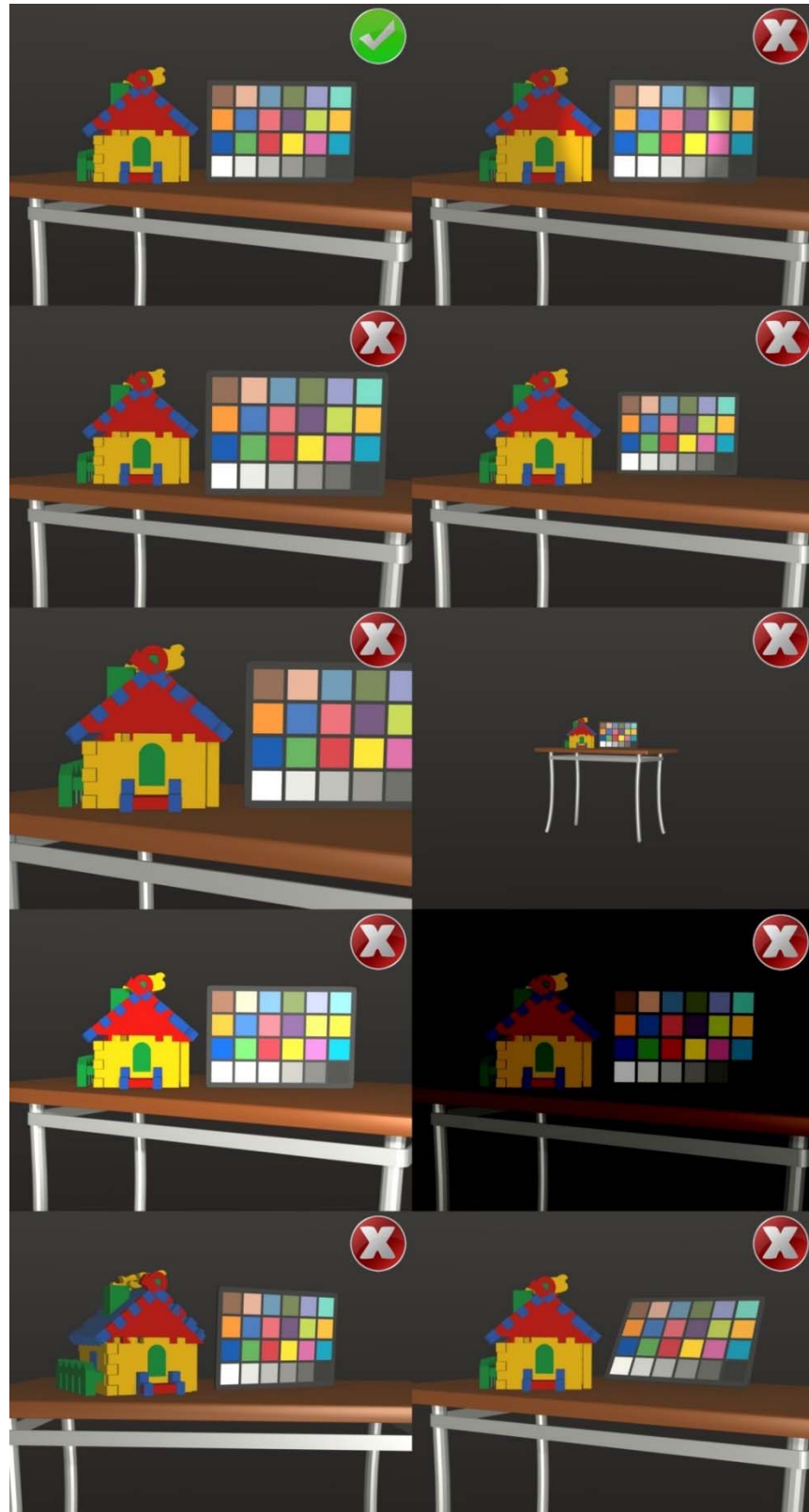
Figure 7: Illustrated photography guidelines. Top row: good image, image with uneven lighting. Second row: chart not in the same region of interest (toy house). Third row: chart not in view, poor framing (too small). Fourth row: over-exposed and under-exposed image. Bottom row: scene not perpendicular to optical axis, and chart is angled.
