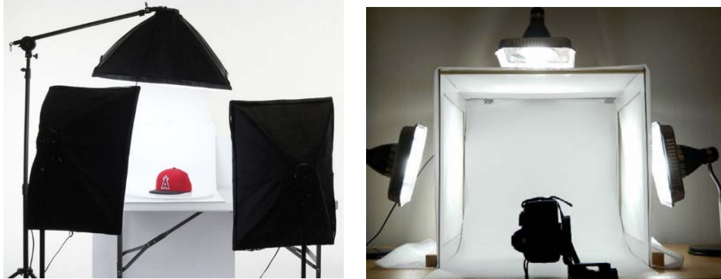
Figure 5: Example of diffuse lighting setups using commercial softbox lighting (left), or a homemade lightbox with diffuse walls (right).
