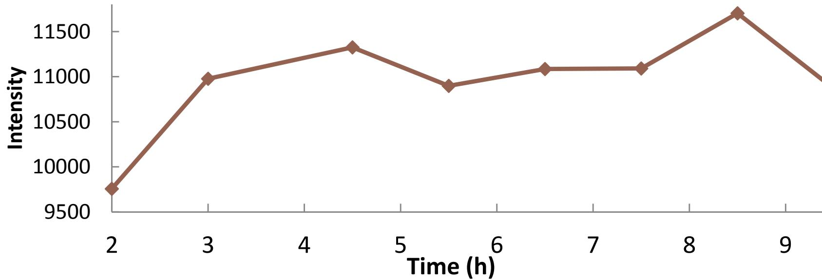
*Dependence of intensity of the gonio-spectrophotometer source on time after turning on.
