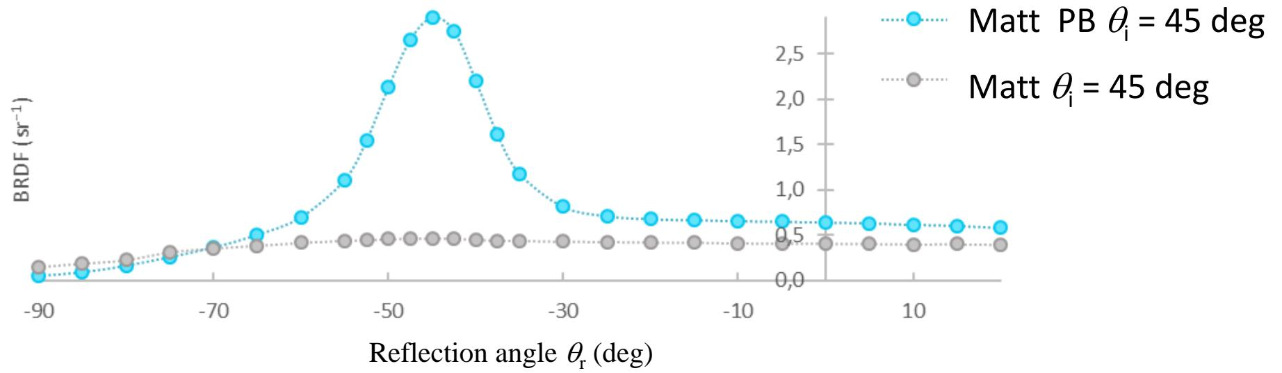
*Dependence of BRDF on reflection angle ( $\theta_i = 45$  deg and wavelength 470 nm).*
