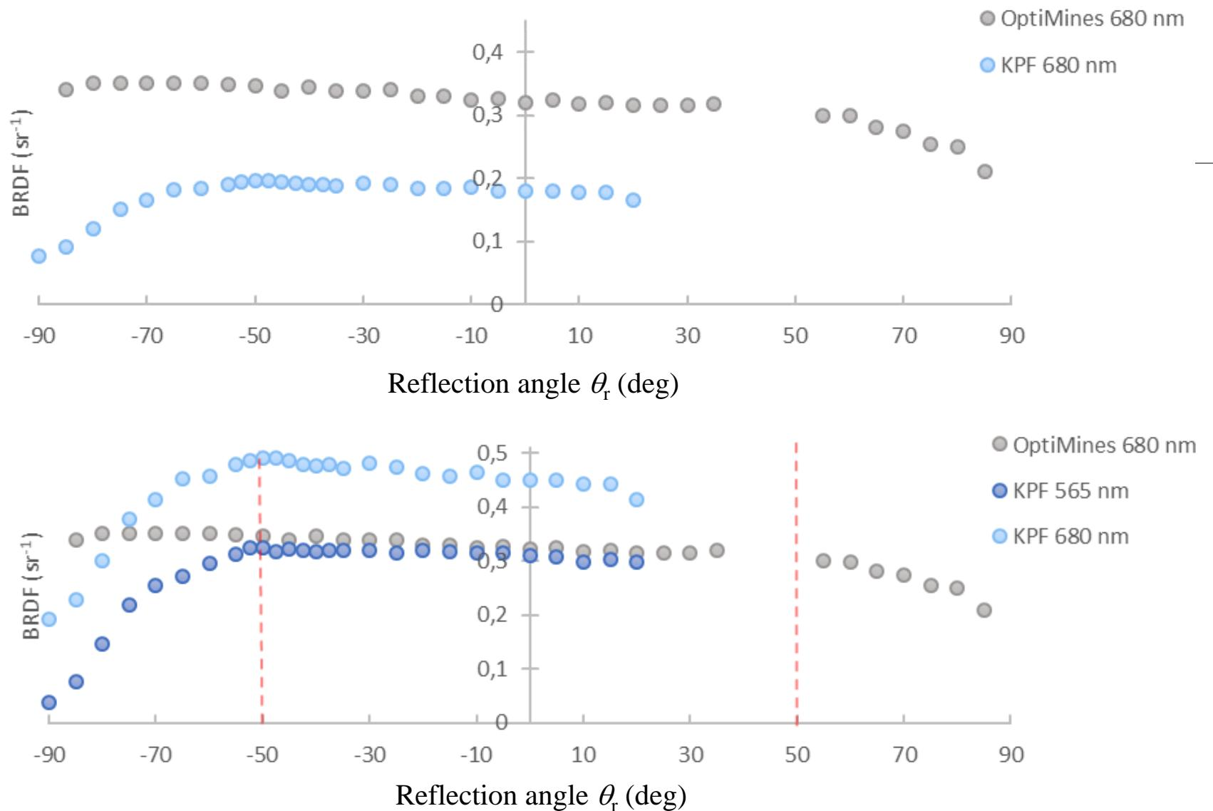
*Comparison of BRDF of the Spectralon obtained from the literature and measured values (up).
