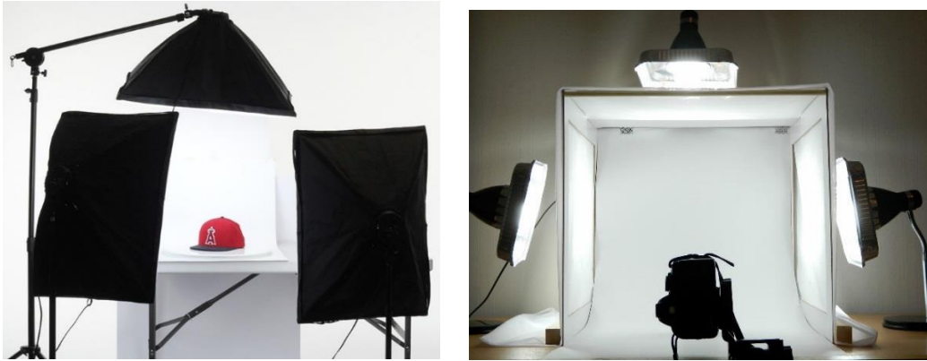
Figure 4: Example of diffuse lighting setups using commercial softbox lighting (left), or a homemade lightbox with diffuse walls (right).
