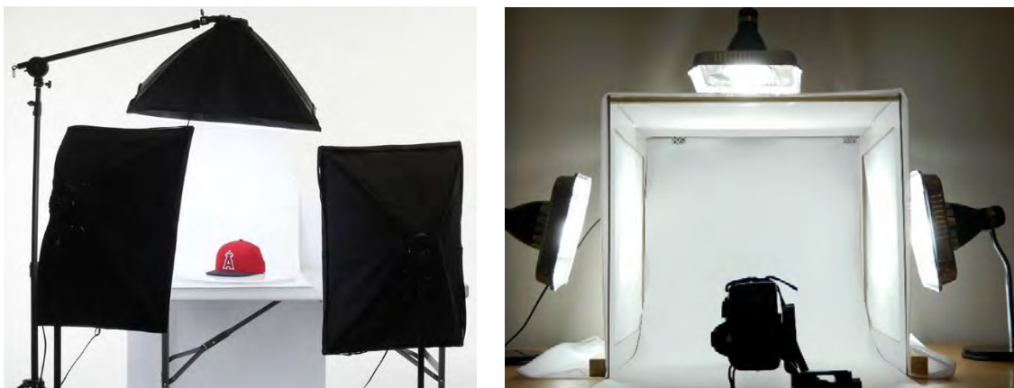
Figure 2. Example of diffuse lighting setups using commercial softbox lighting (left), or a homemade lightbox with diffuse walls (right).
