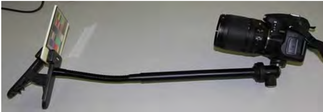
Figure 3. Example fixture used for the side-by-side image capture method.
