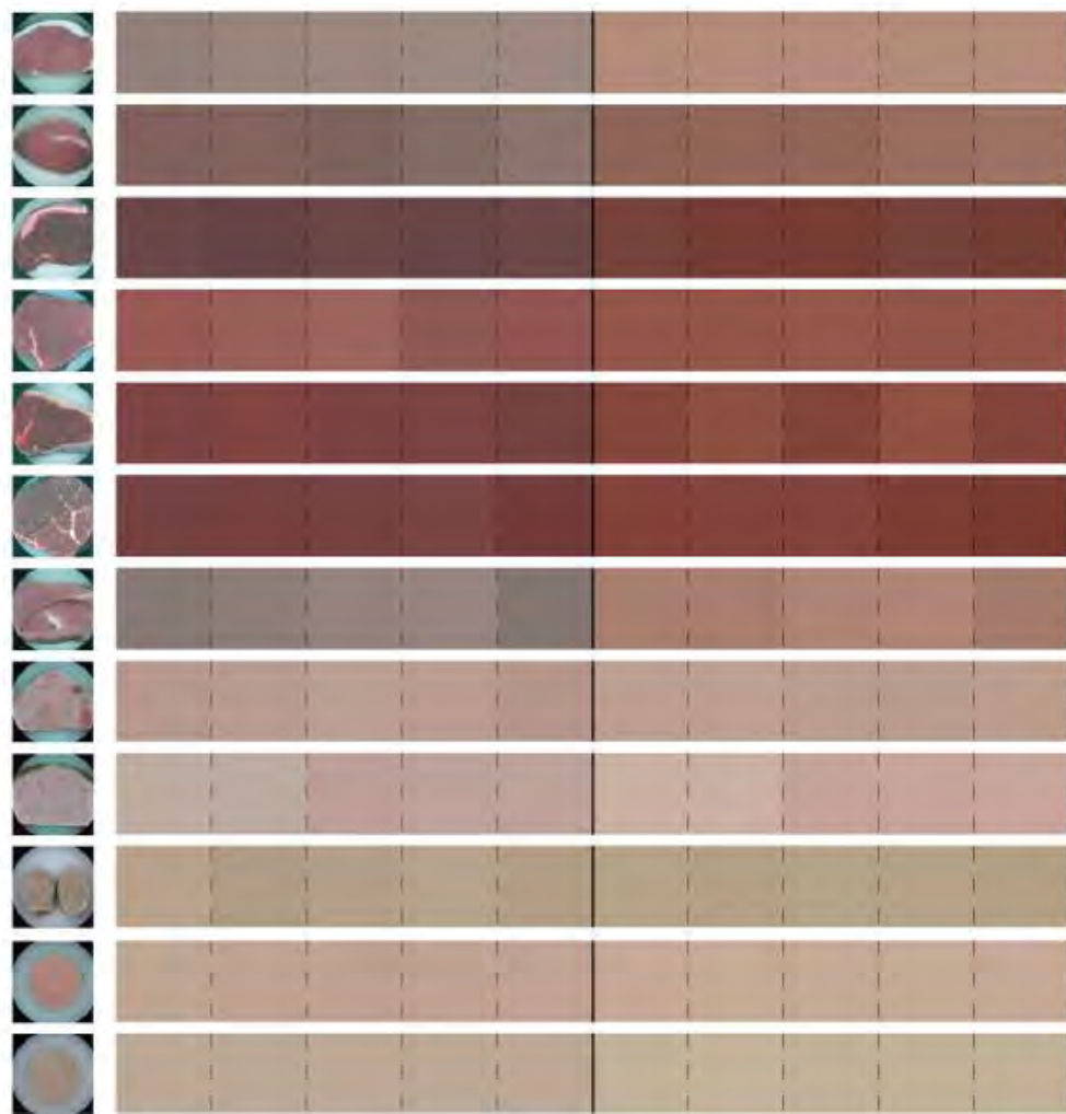
Fig. 4. Colors of the twelve different product types, as evaluated by the two instruments. Here shown in sRGB colors. Left column: Example of product type. Middle column (five blocks): Colorimeter colors. Right column (five blocks): Colors from the vision system. Colors displayed are averages of four site measurements on each sample.
