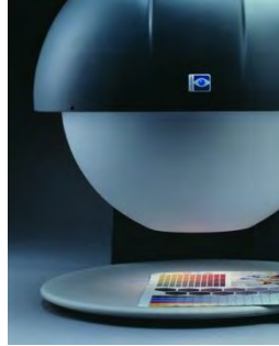
Figure 14. VideoMeterLab 3 : An example of multispectral imaging system (left) and the lighting spectrum (right). [VID 2015]
