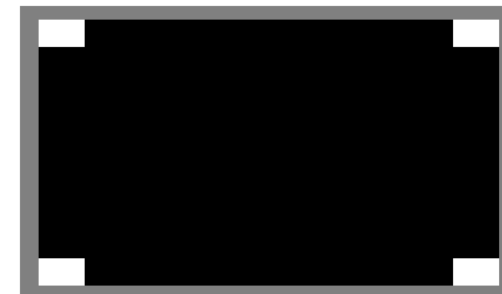
(b) Black center measurement is made with 10% linear boxes in corners
