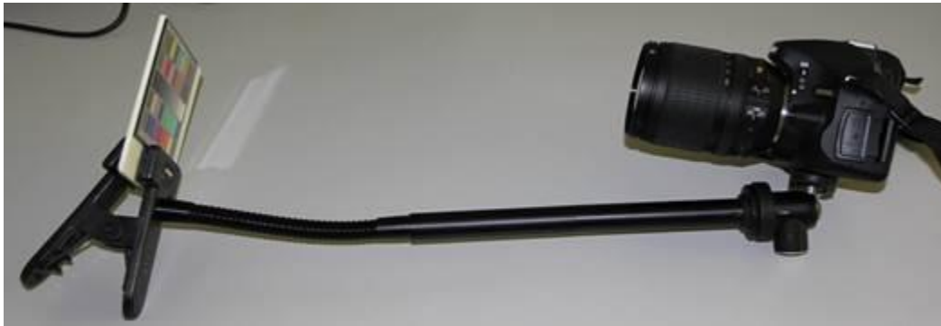
Figure 2. Example fixture used for the side-by-side image capture method.
