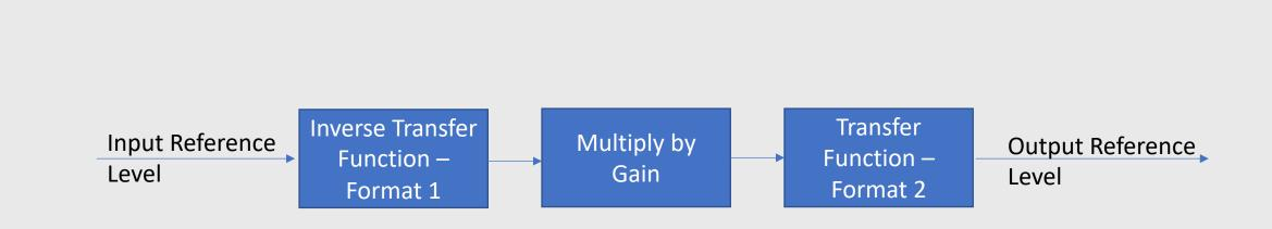
Input and output reference levels and the transfer functions are defined, therefore gain can be calculated
