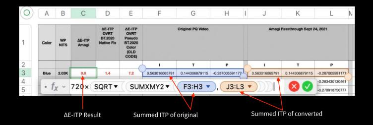
Each sampled ITP Value is multiplied by 720 times the Square Root of the sum of squares of the differences of corresponding values in two arrays
