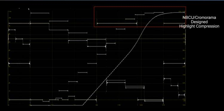
Compressing HDR Highlights to SDR Require Good LUT Interpolation or Accurate Mathematical Conversions
