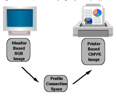
Figure 3 — Profile connection space illustration
